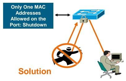
Port security limits MAC flooding attack and locks down port and sends an SNMP trap
